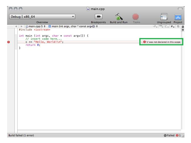
In the rectangle, you can see the compiler error—that Xcode doesn't know what 'c' is. You can also see a message that the build failed, in the lower left corner, and again in the lower right corner, along with a count of the number of errors (1, in this case). (In Xcode 4, the icon is similar, but it appears in the upper-right corner.)
